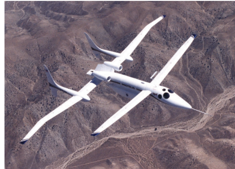
High altitude aircraft will make in situ measurements of stratospheric and tropospheric constituents. Above, the Proteus, and below, the NASA ER-2 have been frequently used in satellite validation.
