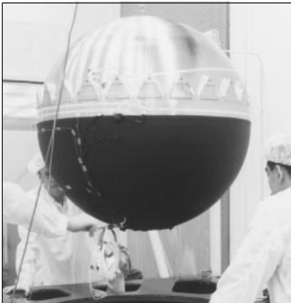
Fuel (Monomethylhydrazine) Tank
