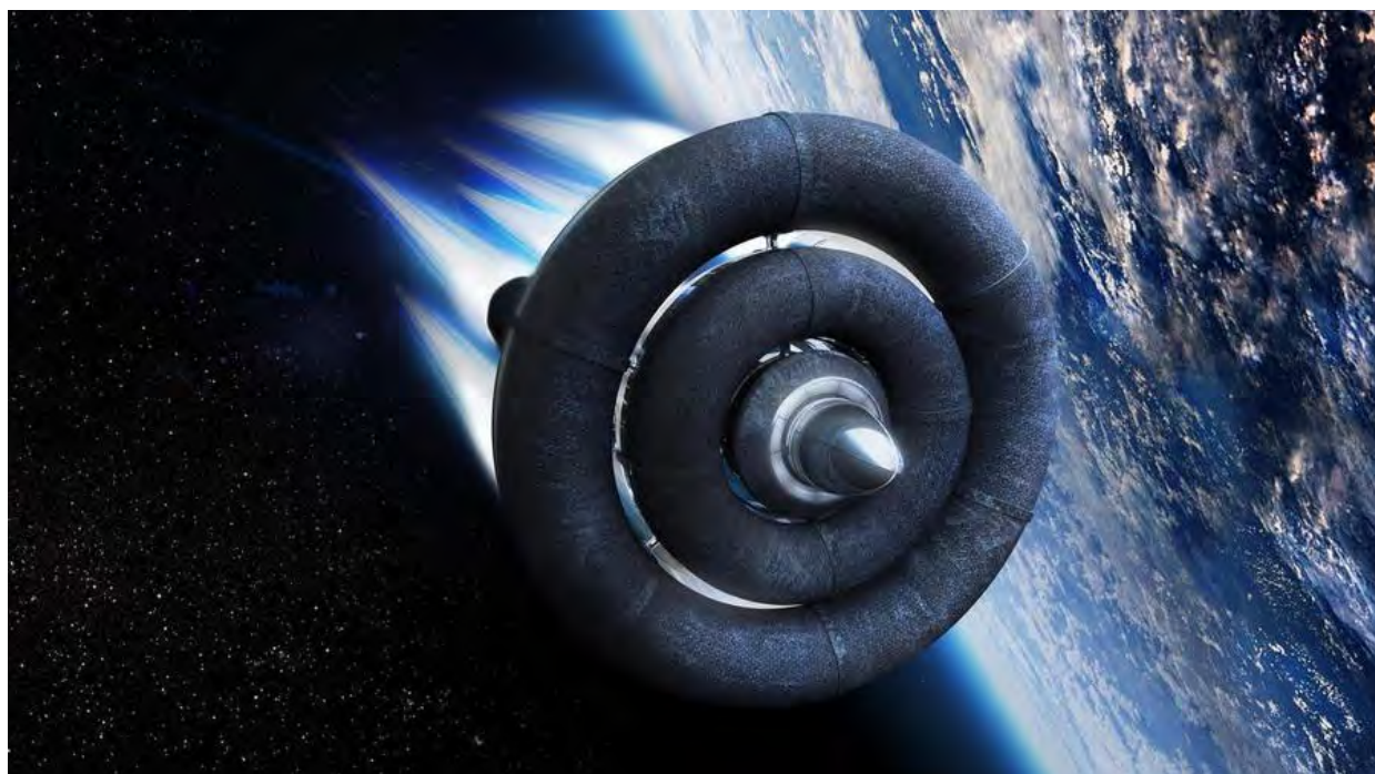
Artist's rendering of Bloostar after release from its balloon. Note the three nested stages and the payload in the center. (Source: Zero2Infinity)
