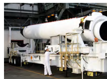
A GEM-60 being prepared for integration on a Delta IV (Orbital ATK)
