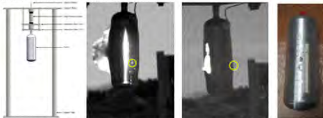
It was able to identify the general opening tendency, and all the openings were evenly distributed along the samples 2.5mm. (0.1in.) Wall thickness (weak point) 19 in. Long, 6 in. Diameter, 6061 Al material
