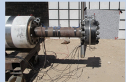
Figure 5. Test fixture for shock wave loading of composite panels
