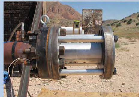
Figure 7. Test fixture for shock wave loading of composite panels
