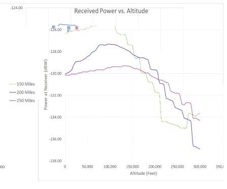
Amplification needed with TPS material added as altitude is increased. Note: TPS material unknown and not included in models shown.
