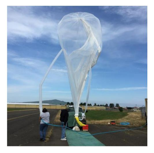
Terminal Velocity Aerospace Reentry Vehicle Drop from stratospheric balloon
