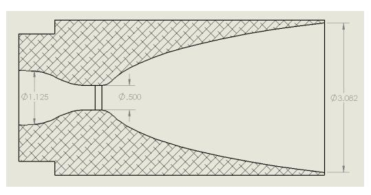
Thrust optimized parabolic (TOP) contour nozzle
