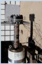
Figure 5. Test fixture for shock wave loading of composite panels
