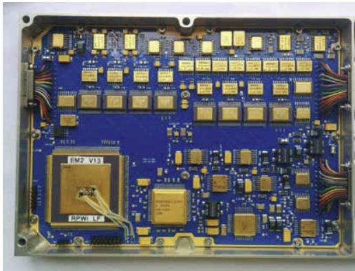
Figure: Left: Engineering model of the LF module for JUICE RPWI which will analyze measurements of the electric and magnetic field. Right: Electronics board of the power supply for the RPWI experiment on JUICE space probe during one of the ground tests. Depicted is engineering model 2B.
