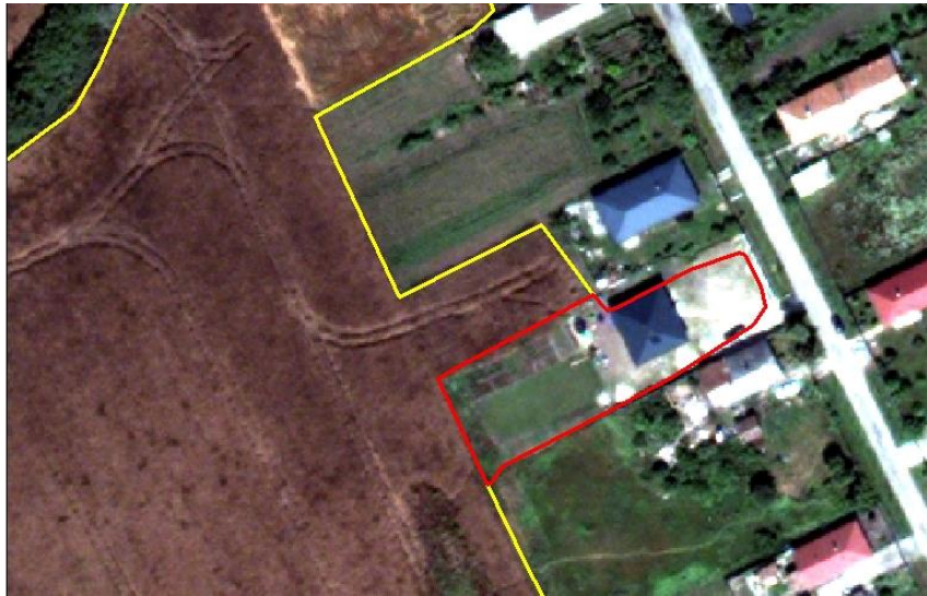
Figure 5.17. Example of the occurrence of non-agricultural land cover features on the reference parcels with causes “Update” – changes of the underlying land were not applied.
