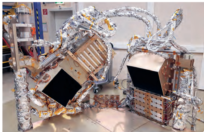
ICI on-ground calibration targets during integration at IABG, Germany.
