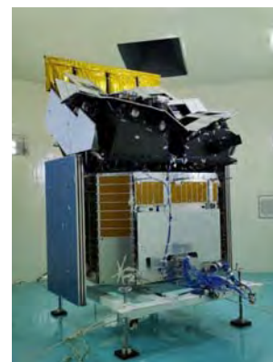
Fig. 7 Structural and thermal model of the EP payload and spacecraft (credit: MicroSat)
