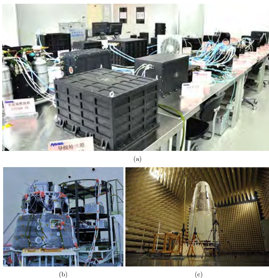
Fig. 3 Test of payloads and satellite (Photo courtesy of SJ-10 mission department) (a) Desktop test of payloads, (b) satellite test of payloads, (c) SJ-10 satellite test
