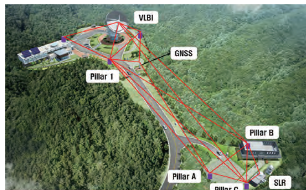
Fig. SC-B-9. Local tie survey pillar installation at Sejong GGOS Site
