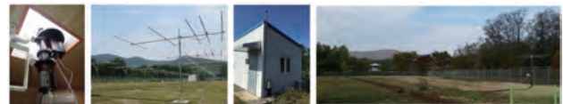
Fig. SC-C-1. All-sky camera, VHF ionospheric radar, GPS scintillation monitor, and meteor radar (left to right)
