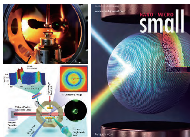
Fig. SC-G-1. Low temperature ESL device (top in left), combination of synchrotron X-ray and Raman scattering devices (bottom in left), and levitation of colloids (right).
