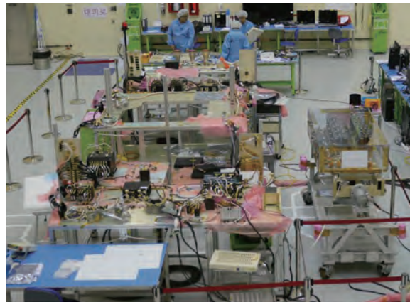
Fig. SC-A-9. Cheollian-2 Electrical Functional Test @ Dummy Wall (image credit: KARI)
