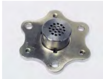
MEMS Acoustic Sensor with AlN as piezoelectric layer
