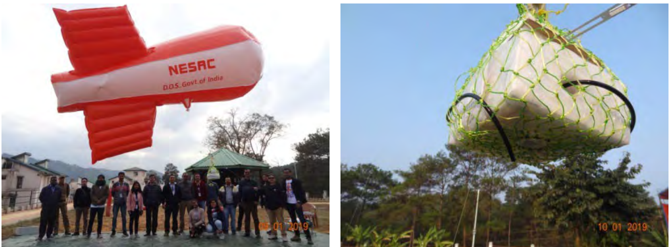
Fig. 1: Hydrogen gas filled tethered balloon (left) and instrumented payload connected with the tethered balloon (right)
