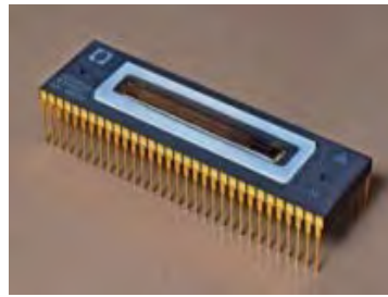
Frame Transfer CCD for OCM 3
