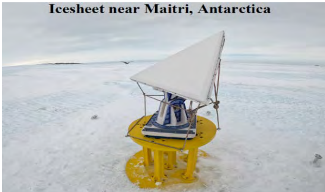
Fig 14: Corner reflectors installed at Antarctica during 39 ISEA
