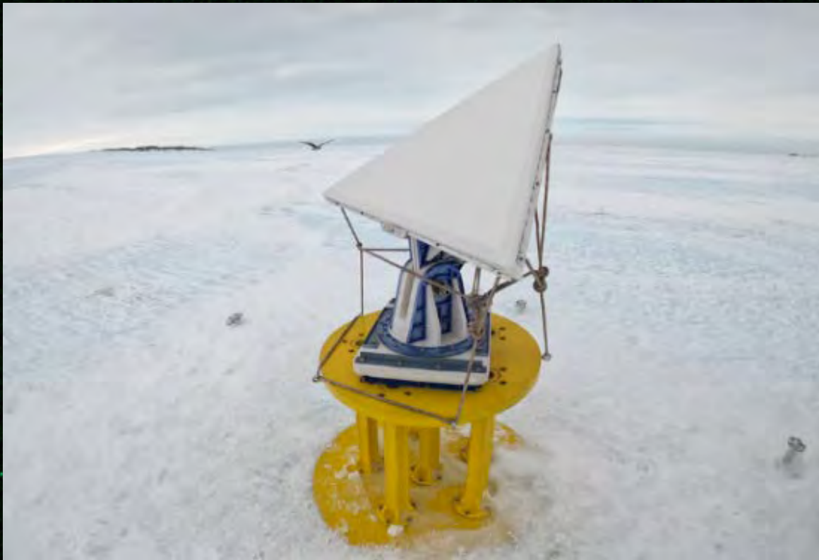
Corner Reflector deployed at icesheet near Maitri Station, Antarctica on January 11, 2020 by 39th Indian Scientific Expedition to Antarctica (ISEA) Maitri team from Space Applications Centre, ISRO and National Centre for Polar and Ocean Research (NCPOR)
