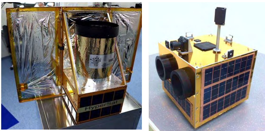
Fig. 4.17. The two different mockups of HyperSat satellite, the generic platform at the left and the platform proposed for UV Satellite at the right, courtesy of Creotech SA
