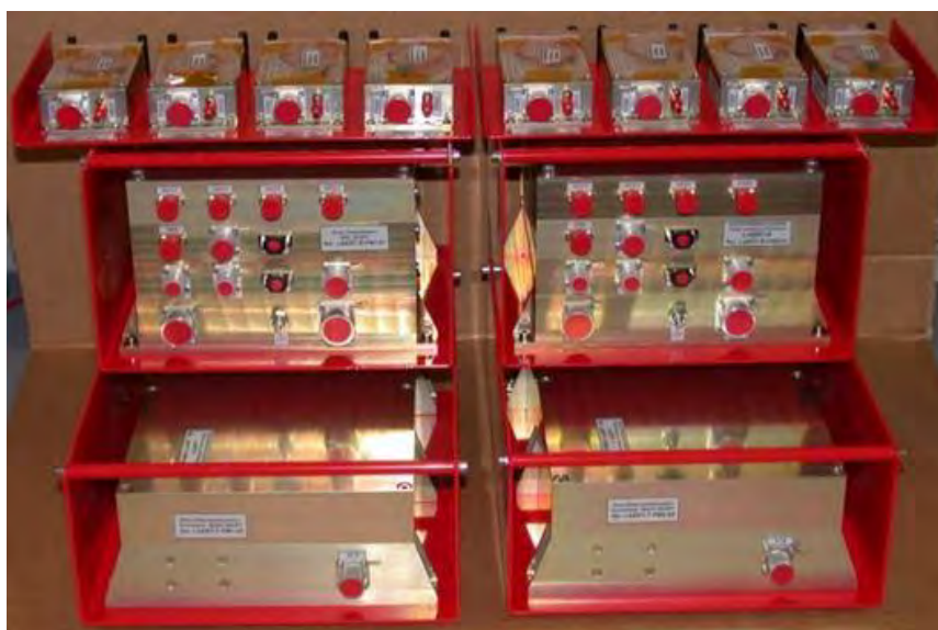
Fig. 4.12. Two sets of Flight Model of LAERT instruments for JONOSONDE mission, © CBK PAN
