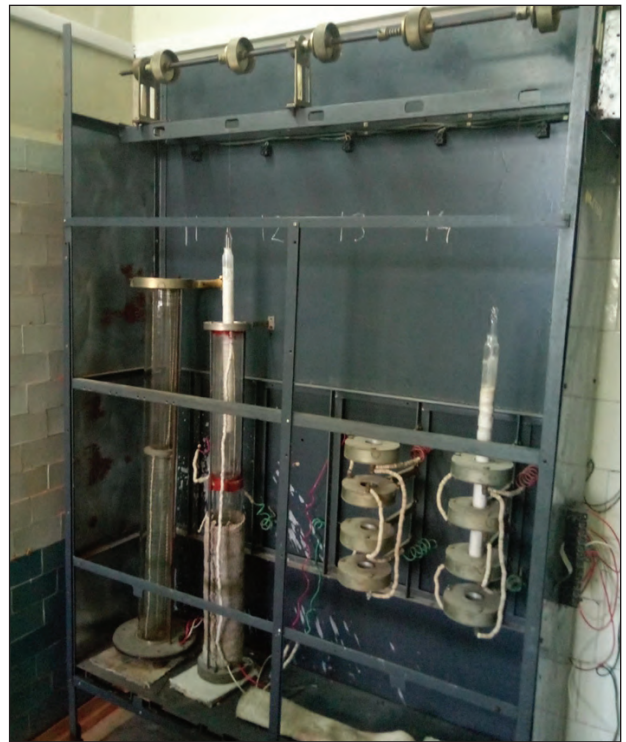
Fig. 8. A facility for zone melting and crystal growth
