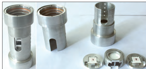
Fig. 4. A view of a manufactured prototype of the detector head (left-hand), and scintillation detectors in their holders (right-hand)
