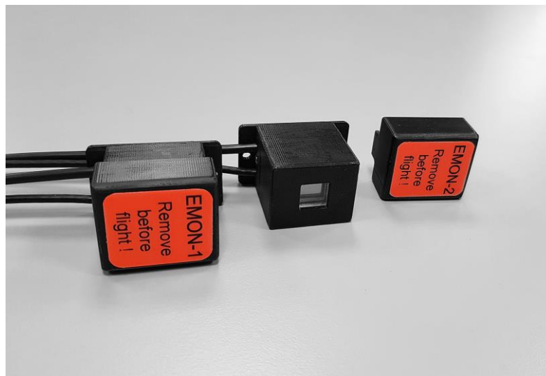
Figure 1.7. A pair of the EMON photo-detectors developed at IEP SAS for NASA-SPB2 mission.
