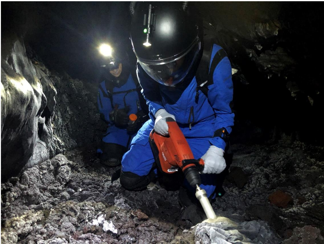
Figure 3.2. Two analog astronauts using a Honeybee Robotics drill to collect geological and biological samples for astrobiology research in a lava cave during a simulated lunar mission at HI-SEAS (Photo credit: Michaela Musilova).
