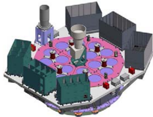
Fig. 2 Main payloads onboard Insight-HXMT . The 18 cylindrical NaI/CsI detectors located around the center are HE, the boxes on the lower left are LE and upper right ME
