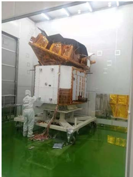
Fig. 10 Assembled satellite before thermal environment test (credit: IMAC)
