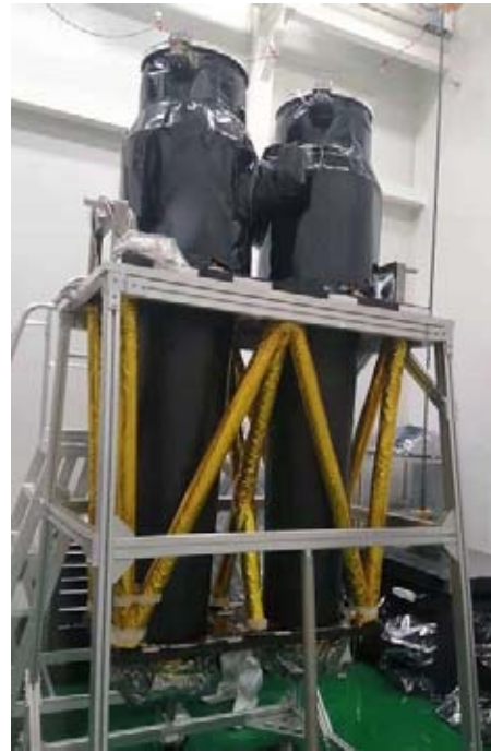
Fig. 8 FXT coated with multiple layers (credit: IHEP, CAS)
