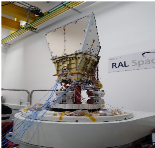
Fig. 5 SXI STM on a shaker table at RALSpace, UK
