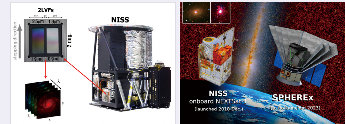
Figure 1. The NISS (right), its Linear Variable Filters (LVFs, upper-left), and an example output spectral map of a galaxy from the LVFs (lower-left). Figure 2. NISS and SPHEREx. The insets show the M33 galaxy and the Orion cloud images captured with NISS's LVFs.
