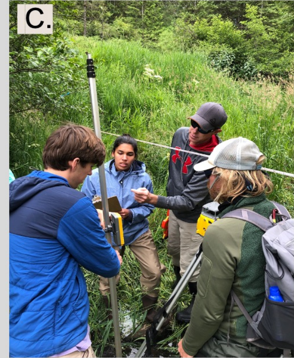
Figure 1. A. Map of study sites (Hangman and Lake Creek) in Northern Idaho. B. Incised channel, resulting from agriculture and land use change at the Lake Creek Treatment Site. C. The team taking stream slope measurements using a laser level.
