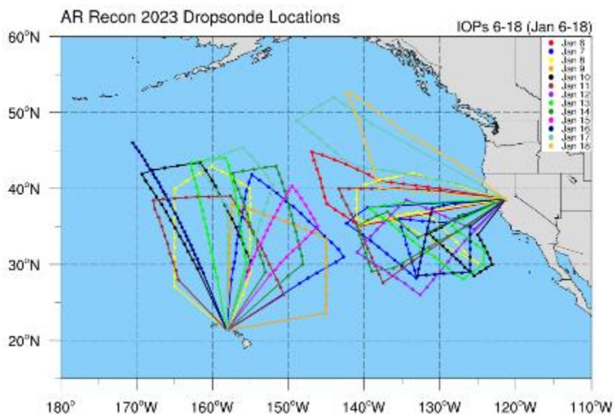
Figure 6-4. Illustration of vertical profiles collected during IOPs 6–18 in AR Recon 2022–2023. Symbols indicate the dropsonde release points and the lines indicate flight tracks. The colors indicate the date of each IOP.
