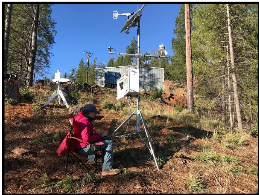
Carly Ellis from CW3E installing a gaging station
