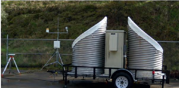
FIG. 5. (right) The snow-level radar, (middle) surface meteorological sensors, and (left) GPS receiver antenna deployed at Pine Flat Dam, California, for the HMT-Legacy project. The 1.2-m diameter radar transmit and receive antennas are placed at the bottom of the sloped antenna enclosures wrapped in marine cover plastic. The sloped covers help shed snow and/or pooling water, which would otherwise inhibit radar performance. The radar electronics and data acquisition computer are situated inside the environmentally controlled cabinet placed between the two antenna enclosures.
