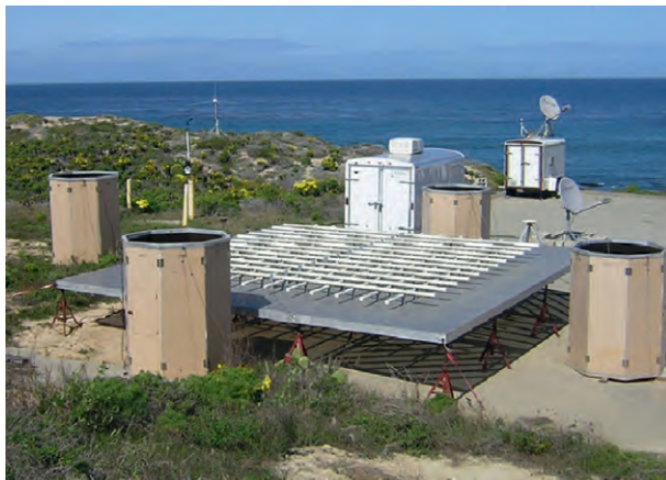
FIG. 8. The ARO installed on San Nicolas Island off the coast of Southern California. The gray panel in the middle of the photo is the frame for the 449-MHz wind profiler coaxial–colinear phased array radar antenna. The octagonal enclosures house the acoustic antennas that are part of the RASS for temperature profiling. The wind profiler and RASS electronics are situated in the environmentally controlled trailer. The site also includes a 10-m meteorological tower (not shown) and a GPS receiver for IWV estimates.
