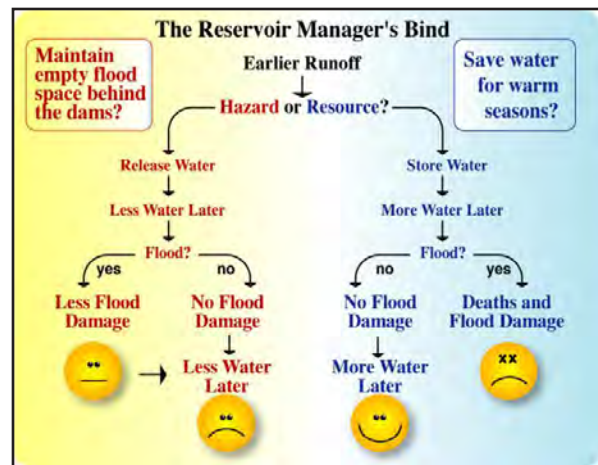
Figure 1. Schematic illustration of possible outcomes associated with early spring runoff depending upon whether the decision is made to release water to preserve flood control space for use in a potential late season flooding storm or to store water in expectation of summertime water-supply demands.
