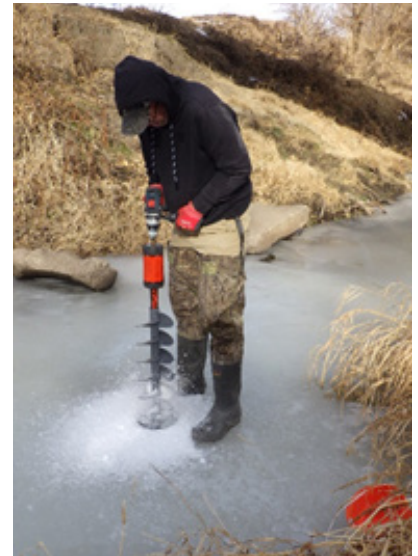
Drilling a hole through the ice to sample the water at Hughes Creek, Nemaha County.
