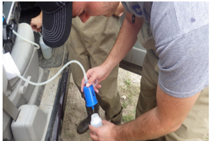
Filtering water sample to be analyzed for various heavy metals.
