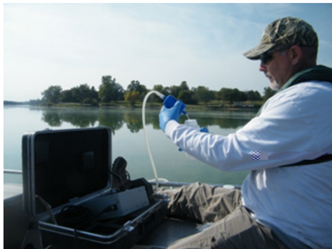
Filtering a water sample to be analyzed for orthophosphorus from Rockford Lake, Gage County.
