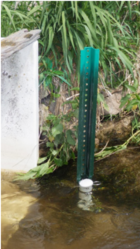
(Above) Temperature sensor deployed in the waters of East Branch Verdigre Creek, Antelope County. (Top right) Downloading temperature data from a sensor.
