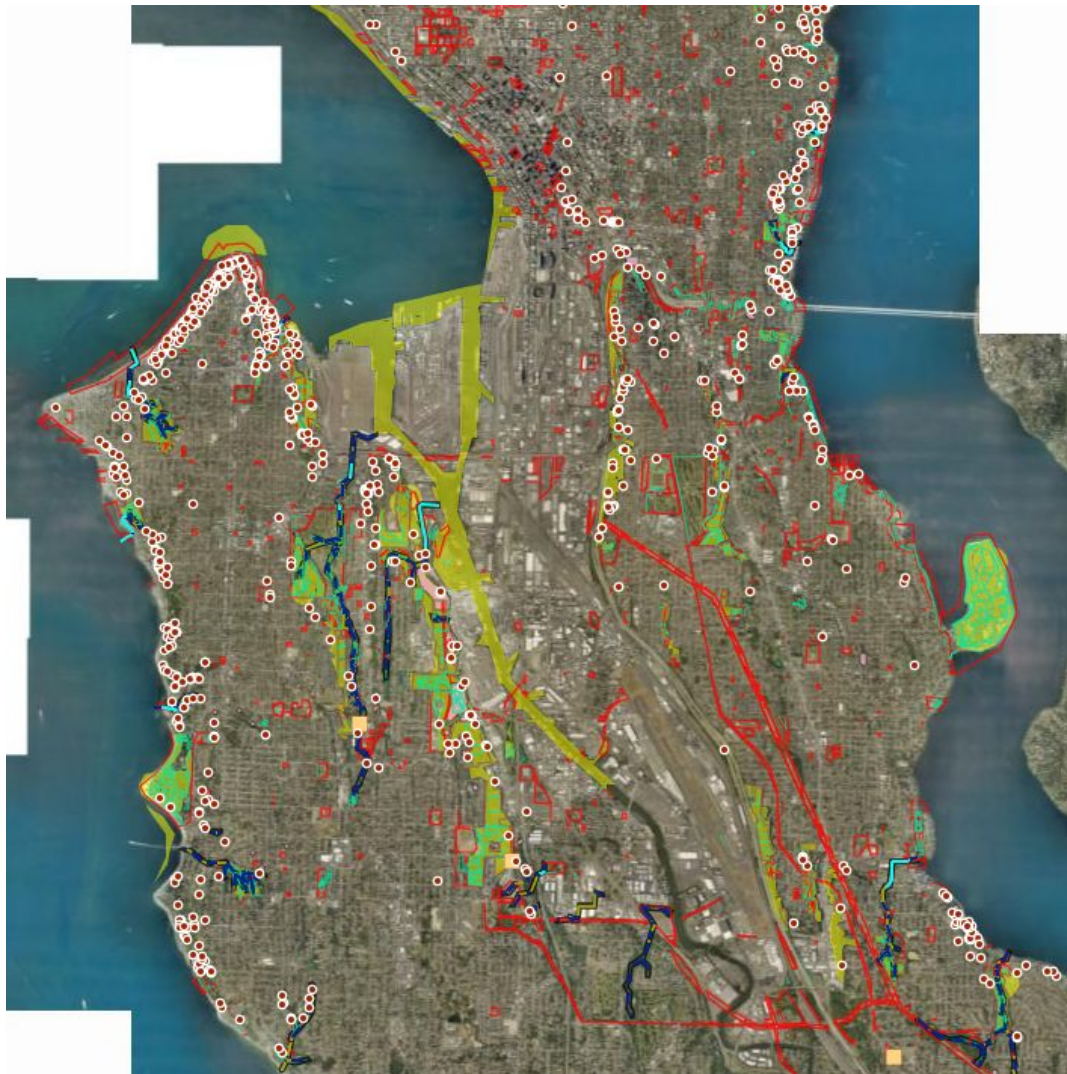
Figure 44: An example of several supplemental data layers that can be utilized to access relevant legal, topographical, or environmental information across an entire study area, or at an individual study site. This analysis informs field data collection and enhances the power of data collected within an individual case study. This example shows city-owned parcel boundaries, environmentally critical areas (including wetlands and wildlife habitats) as well as known landslide locations. The legend is depicted to the right.
