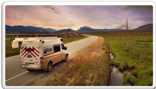
Figure 7: Pavement Data Collection Van Located on the Dalton Highway.
