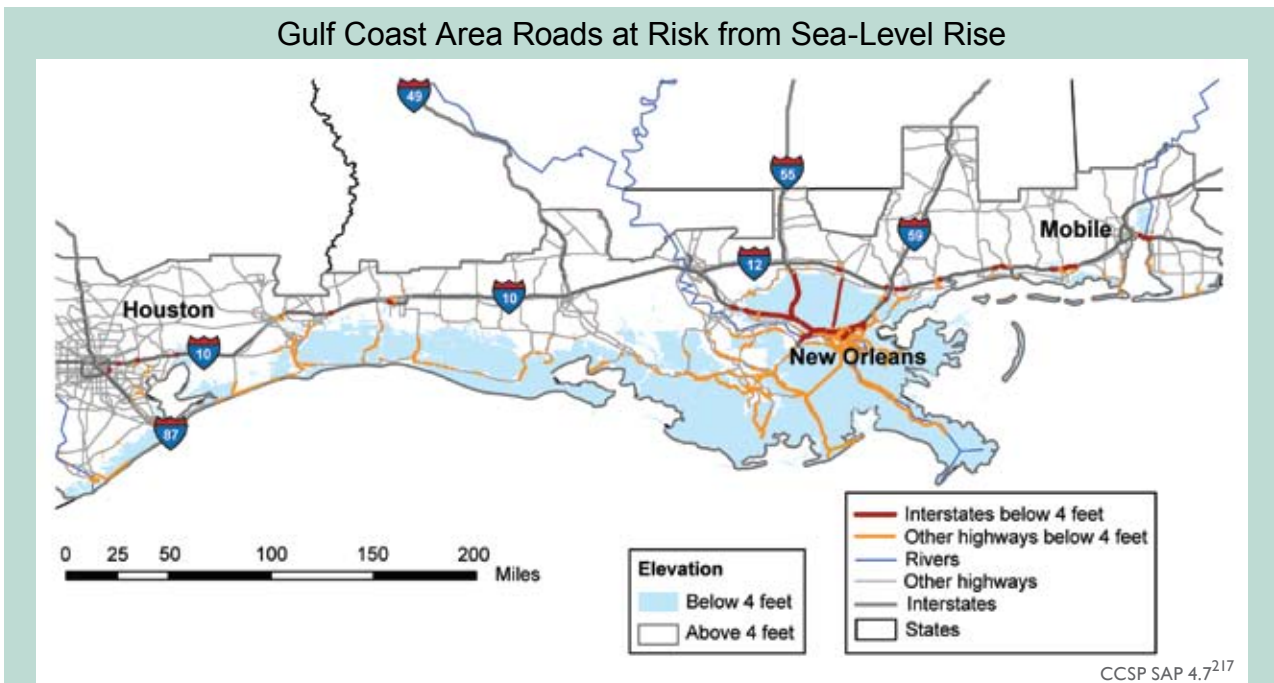
Within 50 to 100 years, 2,400 miles of major roadway are projected to be inundated by sea-level rise in the Gulf Coast region. The map shows roadways at risk in the event of a sea-level rise of about 4 feet, within the range of projections for this region in this century under medium- and high-emissions scenarios. 91 In total, 24 percent of interstate highway miles and 28 percent of secondary road miles in the Gulf Coast region are at elevations below 4 feet. 217
