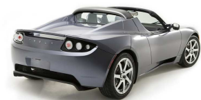
Figure 20.22. Tesla Roadster: 15 kWh per 100 km . www.teslamotors.com .
