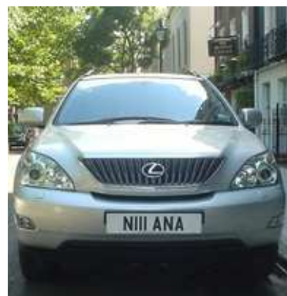
Figure 20.1. This chapter's starting point: an urban luxury tractor. The average UK car has a fuel consumption of 33 miles per gallon, which corresponds to an energy consumption of 80 kWh per 100 km. Can we do better?
