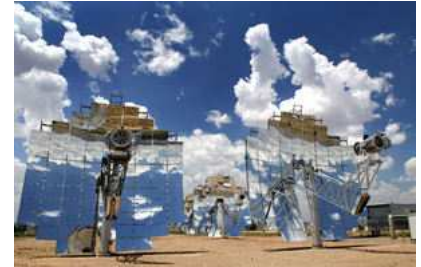
Figure 25.3. Stirling dish engine. These beautiful concentrators deliver a power per unit land area of 14 \text{ W/m}^2 . Photo courtesy of Stirling Energy Systems. www.stirlingenergy.com
