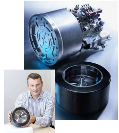
Figure 20.18. A flywheel regenerative-braking system. Photos courtesy of Flybrid Systems.
