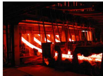
Figure H.1. Continuous casting of steel strands at Korea Iron and Steel Company.
