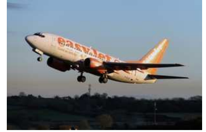
Figure C.11. Boeing 737-700: 30 kWh per 100 passenger-km. Photograph © Tom Collins.
