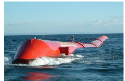
Figure 12.1. A Pelamis wave energy collector is a sea snake made of four sections. It faces nose-on towards the incoming waves. The waves make the snake flex, and these motions are resisted by hydraulic generators. The peak power from one snake is 750 kW; in the best Atlantic location one snake would deliver 300 kW on average. Photo from Pelamis wave power www.pelamiswave.com .
