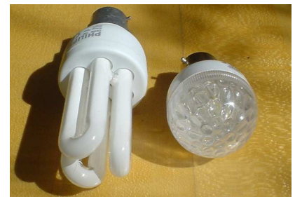
Figure 9.4. Philips 11 W alongside Omicron 1.3 W LED bulb.
