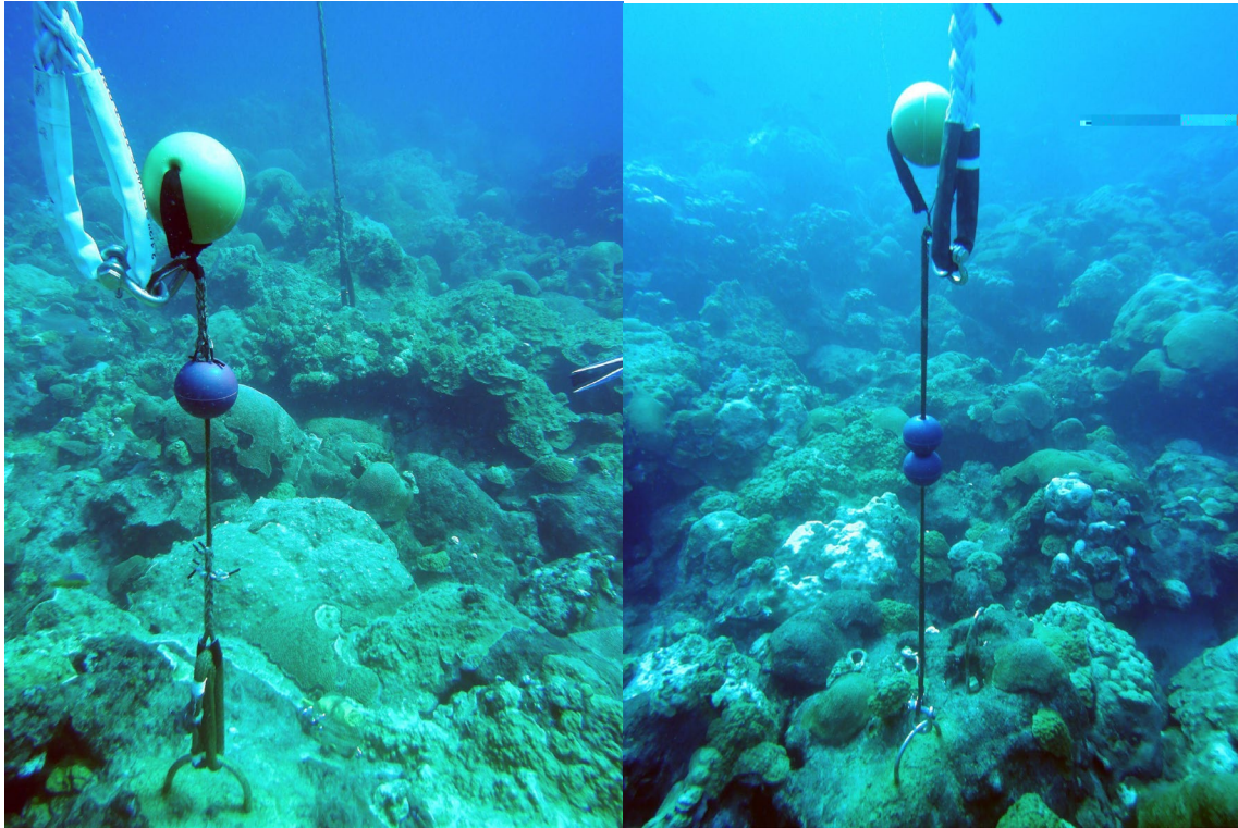
Figure 4. New mooring design prototypes installed at FGBNMS using subsurface buoys and a Dyneema shackle (left) vs the original metal shackle (right) to compare effectiveness. Photos: Josh Harvey/CPC Inc.
