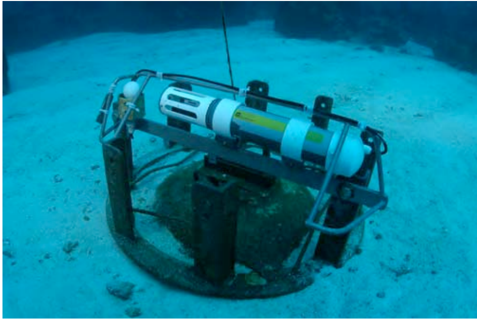
Figure 6. Water quality instrument rack at West Flower Garden Bank prior to Hurricane Rita. Photo credit: FGBNMS/Schmahl
