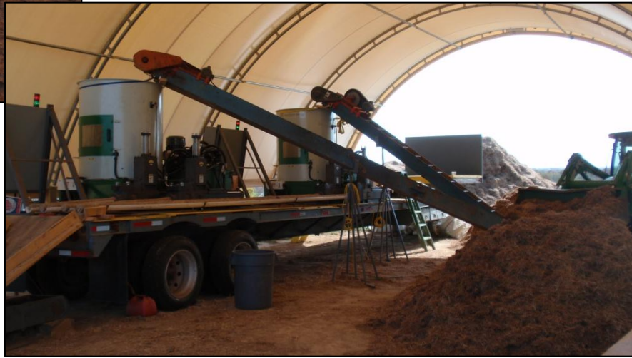
Figure 17. Conveyors take ground switchgrass to briquetters mounted on a trailer. Photo by Dr. Ray Smith, 2012.
