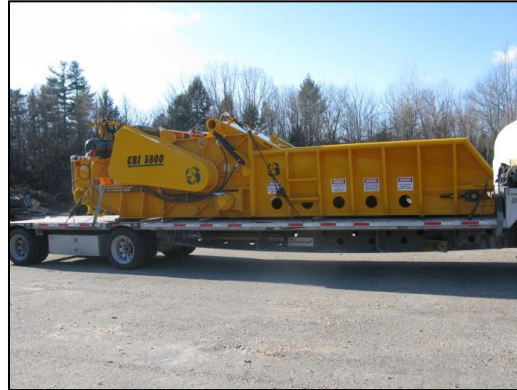
Figure 22. Continental Biomass Industries, Inc. 5800T Grinder – trailer mounted. Picture courtesy of CBI, Inc.
