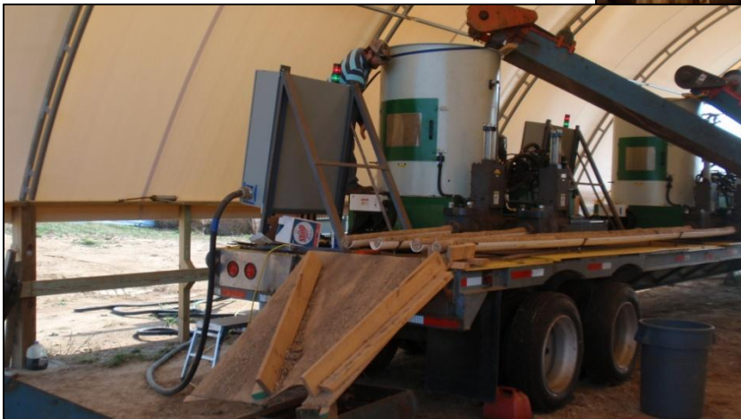
Figure 18. Briquetters from Biomass Briquette Systems, LLC. Photo by Lee Carol Greenwell, 2012.
