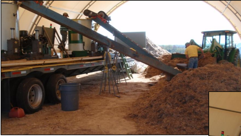
Figure 16. University of Kentucky's switchgrass processing equipment includes a tub grinder, tractor with front-end loader, two conveyors, and two briquetters mounted to a trailer. Photo by Dr. Ray Smith, 2012.
