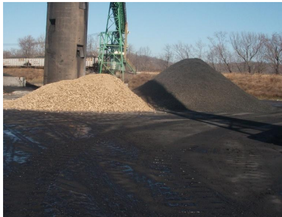
Ground switchgrass ready to be mixed with coal
