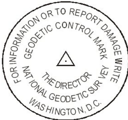
National Geodetic Survey New Geodetic Control Disk
