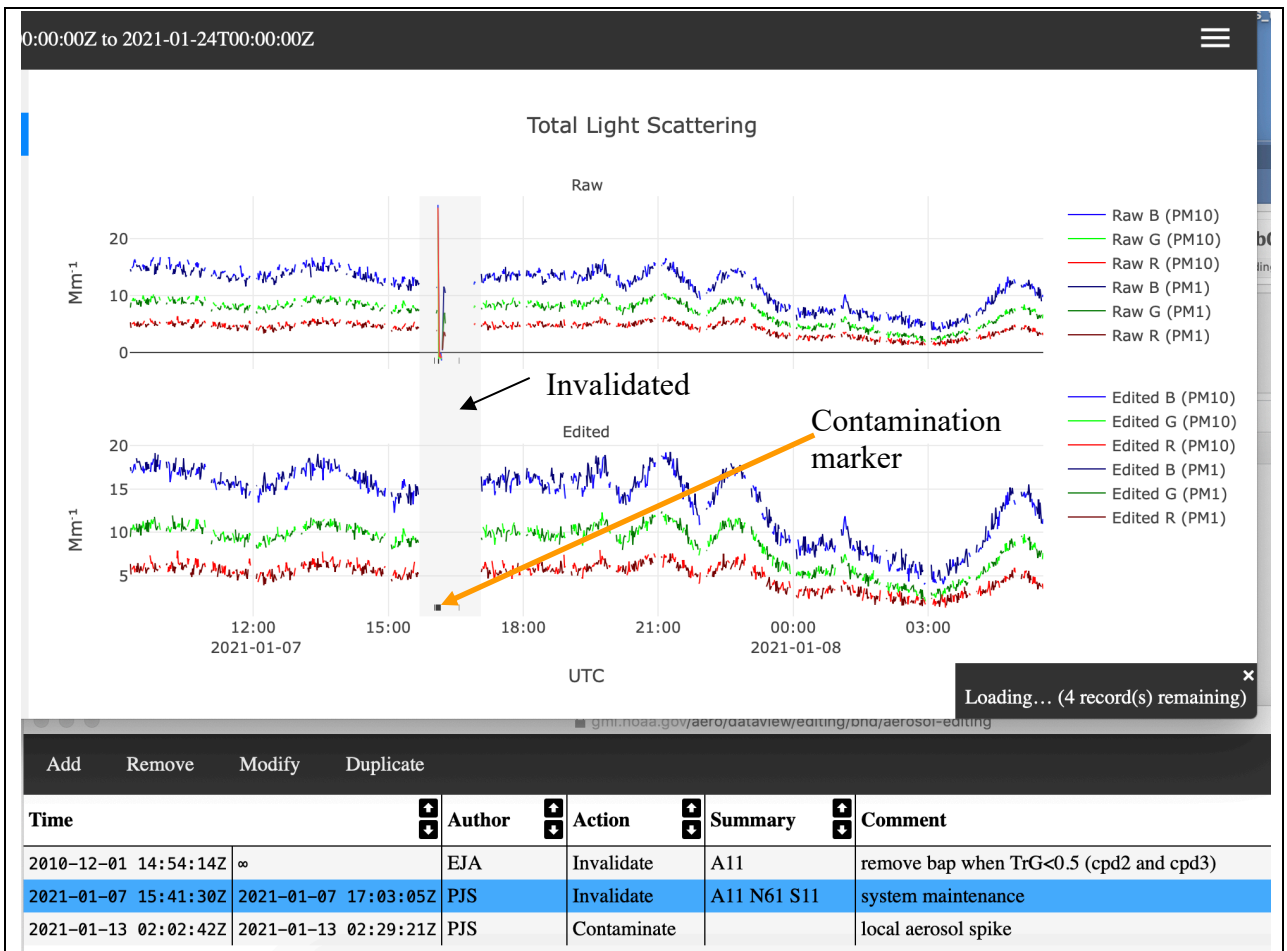
Figure 3 Vertical gray shading in plot shows time range of selected edit (line highlighted in blue in Edit Directives window, seen below plots). Display mode is ‘Edit’ so you see both the raw and edited data. Orange arrow points to flag indicator for data marked as contaminated.
