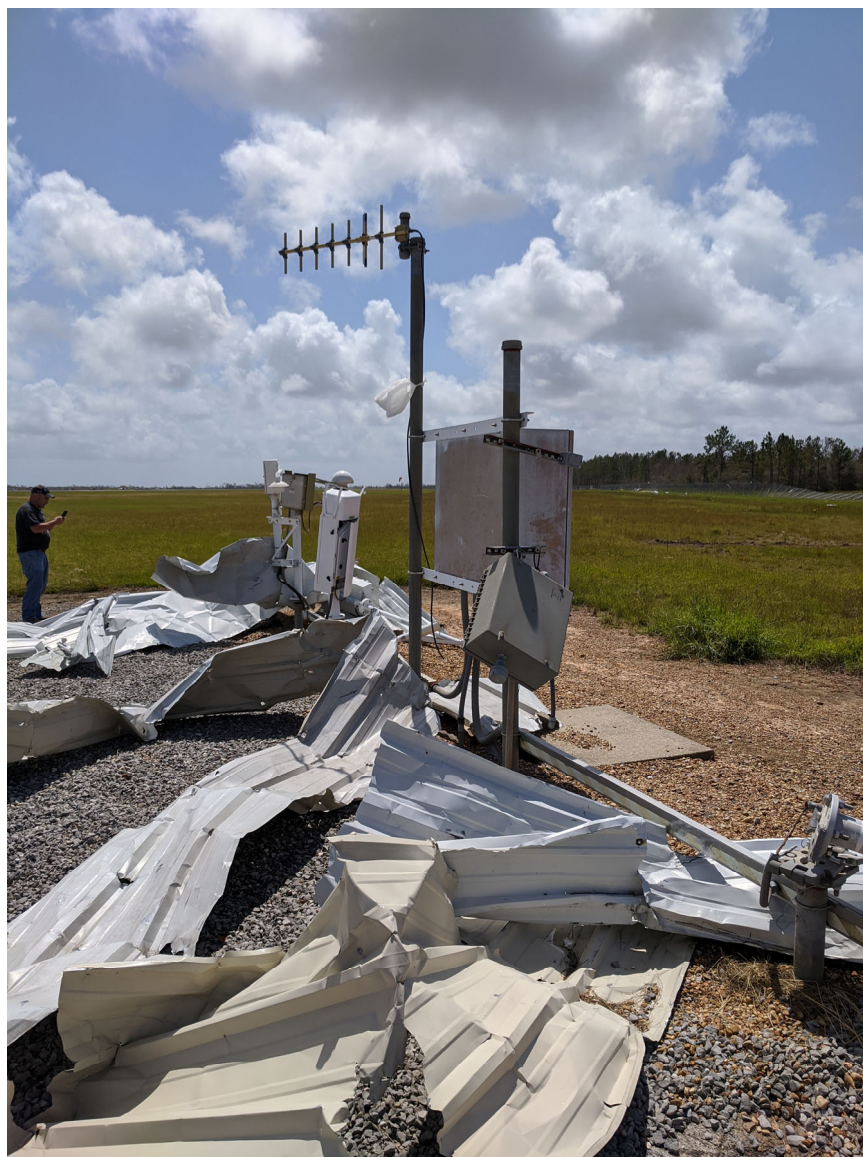
Figure 4. The Lake Charles NWS ASOS surface weather measuring instruments after Hurricane Laura. Image courtesy of David Fontenot, NWS Lake Charles WFO.
