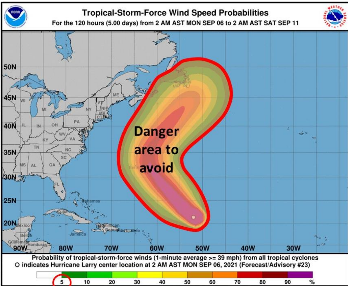
Figure 64: Using the Tropical-Storm-Force Wind Speed Probability graphic as a ship routing tool.
