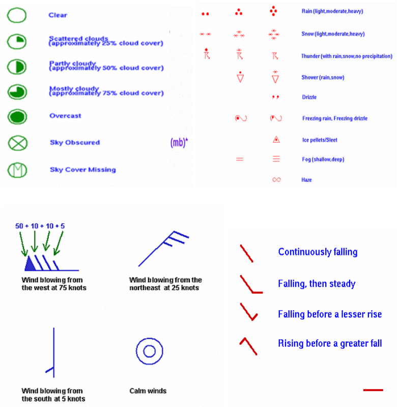
Figure 1. Sample Station Plot and legends to decode present weather, pressure tendency, wind direction and speed and skycover.
