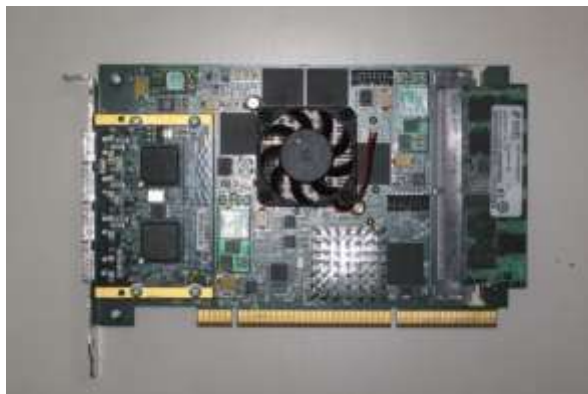
FPGA board H101-PCIXM manufactured by Nallatech
