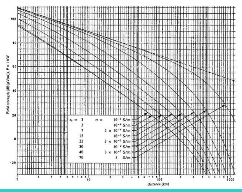
Norton provided a graphical method of modelling the surface wave around a homogeneous smooth earth by means of a complex attenuation function.
