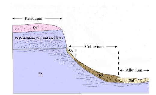
Figure B. Idealized cross-section of hillslope and suficial units formed on bedrock with a sandstone cap and vertical sandstone rock face. Note the difference in colluvium (Qc) and the colluvial accumulation zones (Qca). Here the **Qca** intersects a broader channel occupied by **Qal.** (Modified from Newell, 1978).
