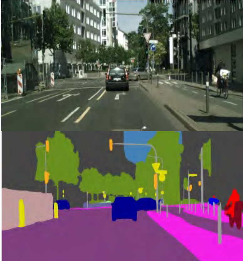
Selected pixel-level features segmented by the PSPNet algorithm for each GSV image
