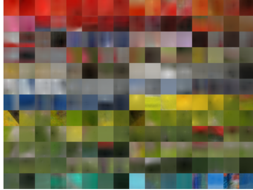
Figure 3. Semantic textons. A visualization of leaf nodes from one tree (distance d = 21 pixels). Each patch is the average of all patches in the training images assigned to a particular leaf node l . Features evident include color, horizontal, vertical and diagonal edges, blobs, ridges and corners. Associated with each semantic texton is a learned distribution P(c|l) , used to give the rough local segmentation of Figure 1(c).
