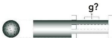
An uneven particle distribution within the beam diameter makes the result, even with a known aperture ratio, uncertain.
