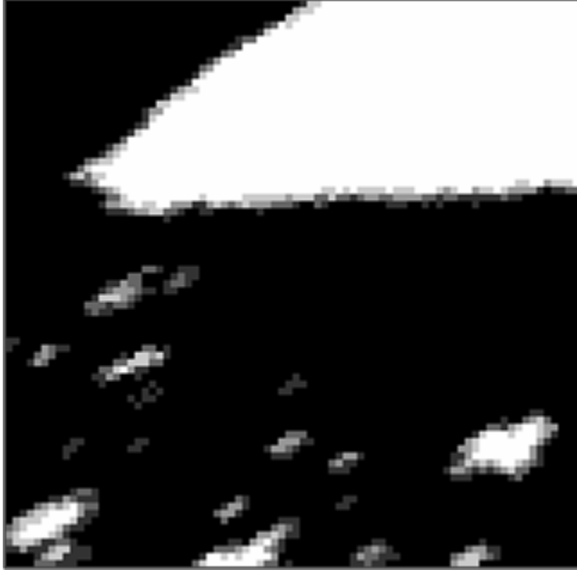
Figure 8. Five-day composite of inland water mask in MOD10A1. The inland water mask, bit 0 of NDSI_Snow_Cover_Algorithm_Flags_QA, was extracted for 7-11 January 2003 and composited. In this composite image of the southern end of Lower Red Lake in Minnesota, black is land on all five days and white is lake on all five days, shades of gray are where the cell was 'not lake' on all five days. Shades of gray from light to dark show where lake was mapped to the cell on from 1 to 4 days in the period. Shades of gray represent the geolocation wobble of lakes.
