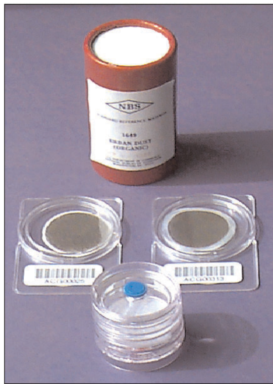
Fig. 24. NIST Standard Reference Material 1649a (“urban dust”). Photograph of the bulk reference material and derived “filter samples” for QA of atmospheric elemental carbon (EC). ^{14}\text{C} data listed indicate the mass fraction (%) of biomass-C in the several chemical fractions [29, 62].
