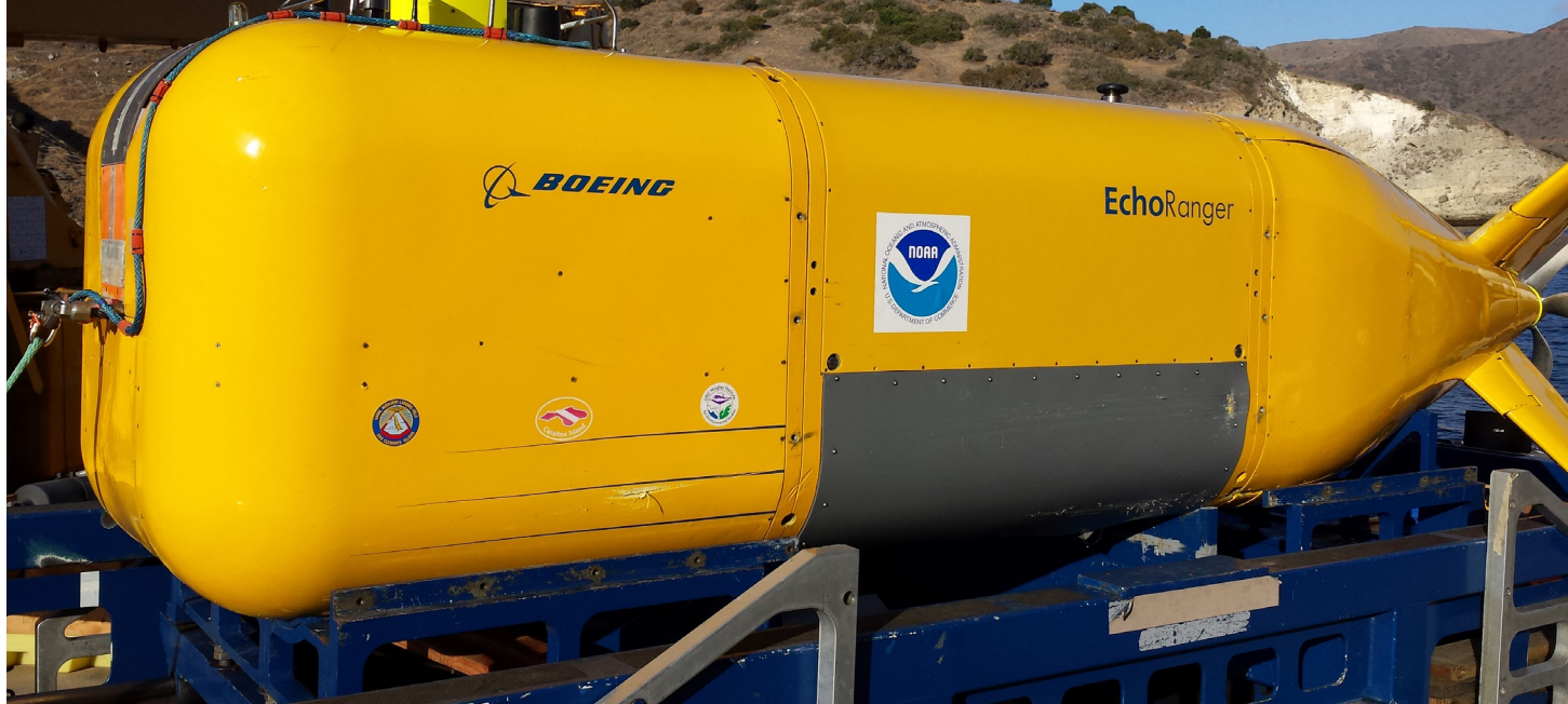
Echo Ranger is a large displacement AUV, 18.5 feet long, with a 150-nautical-mile range and maximum speed of six knots. The vehicle can be deployed from shore and allows increased payload for sensors and longer mission endurance. Credit: Boeing.
