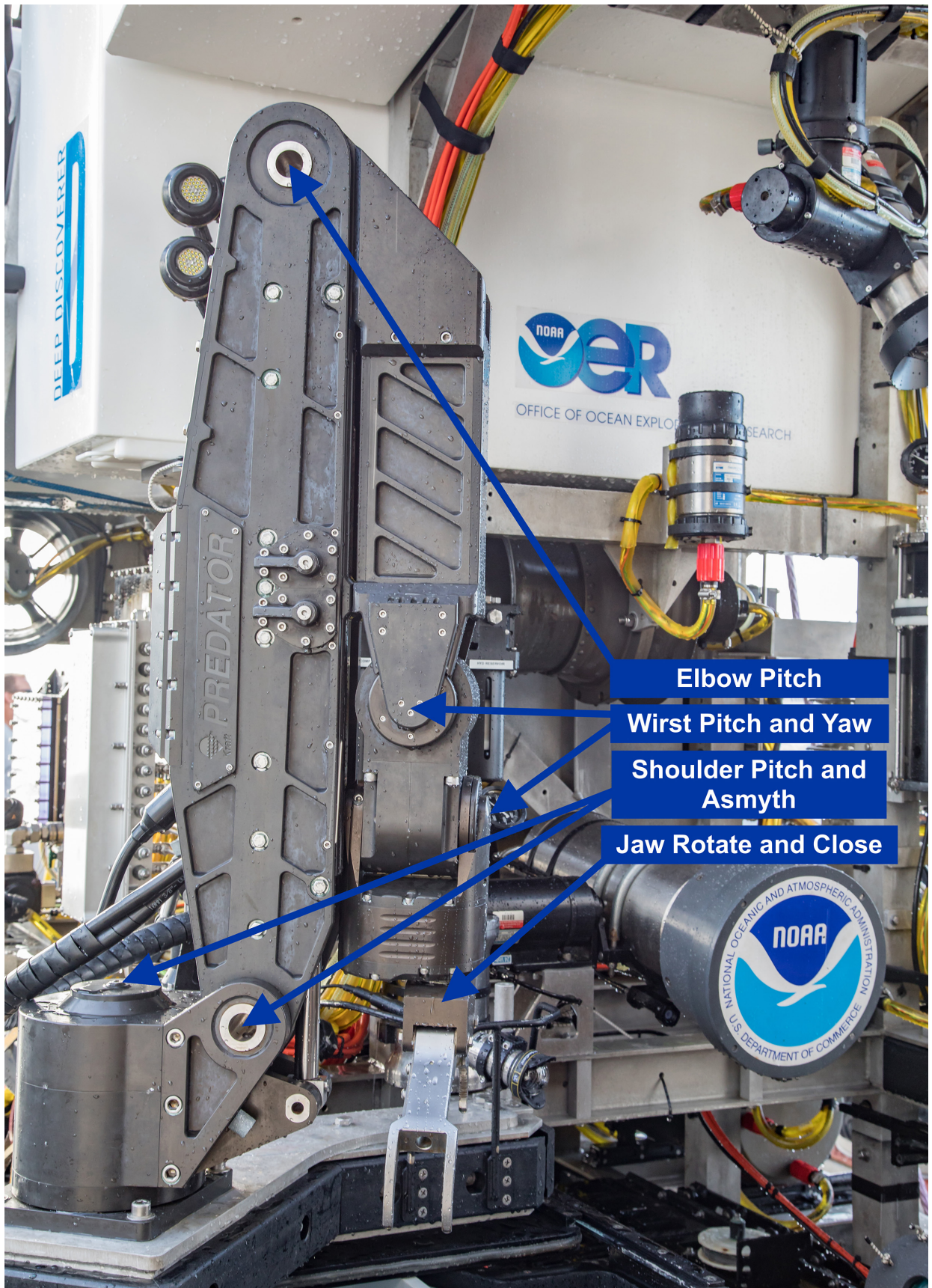
Remotely operated vehicle Deep Discoverer's manipulator arm, labeled. Image courtesy of Art Howard, GFOE; edited by Jeffery Laning, GFOE. http://oceanexplorer.noaa.gov/oceanos/explorations/ex1702/logs/feb28/media/d2arm.html
