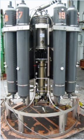
A CTD (Conductivity, Temperature, Depth). Image courtesy NOAA OER.
