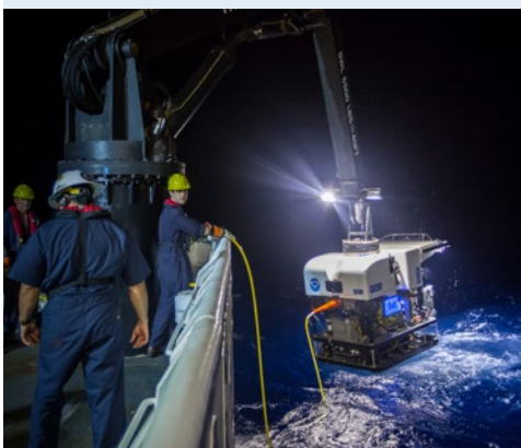
Remotely operated vehicle Deep Discoverer being recovered. Image courtesy of NOAA OER, 2016 Deepwater Exploration of the Marianas. http://oceanexplorer.noaa.gov/okeanos/explorations/ex1605/logs/may1/media/1605rovrecovery.html
