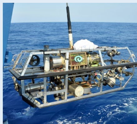
Argus acts as a stabilizing platform for Hercules , following the ROV into the water. Image courtesy of Ocean Exploration Trust. http://oceanexplorer.noaa.gov/technology/subs/hercules/argus.html
