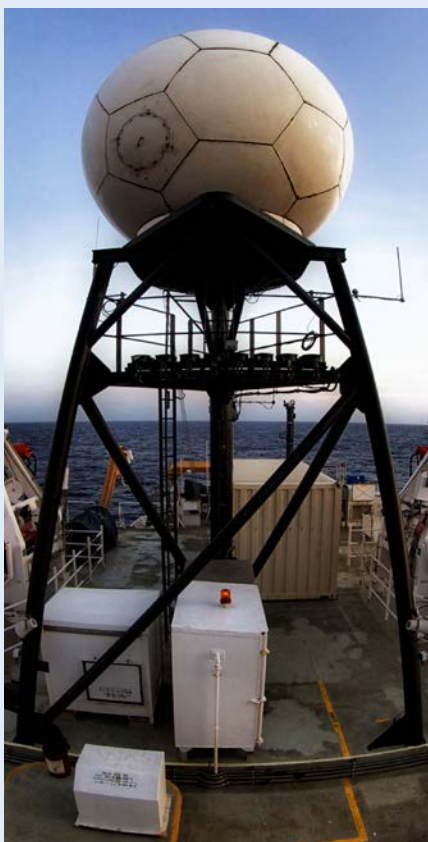
The VSAT (large dome; stands for "Very Small Aperture Terminal") is the critical piece of infrastructure that makes telepresence possible. Image courtesy NOAA OER, Deepwater Wonders of Wake http://oceanexplorer.noaa.gov/okeanos/explorations/ex1703/logs/mar16/welcome.html
