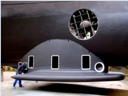
The sonar gondola beneath Falkor's bow. A big challenge for sonar systems on most ships is bubbles. As a ship moves faster, or encounters heavy seas, bubbles formed at the surface wash down the hull, where they can interfere with the sending and receiving of sonar signals. To overcome this issue, Falkor's sonar systems are installed on the bottom of a streamlined platform. The sonar systems are embedded into the bottom surface of this gondola, where they are isolated from bubbles, which pass between the hull and the top of the gondola. https://schmidtocean.org/technology/sea-floor-mapping/
