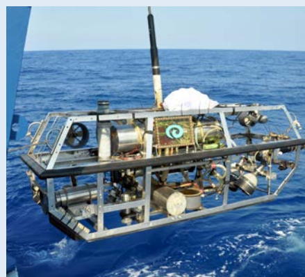
Argus acts as a stabilizing platform for Hercules, following the ROV into the water. Image courtesy of The Ocean Exploration Trust. http://oceanexplorer.noaa.gov/technology/subs/hercules/argus.html
