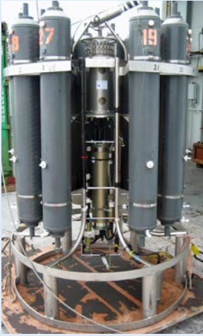
A CTD (Conductivity, Temperature, Depth). Image courtesy NOAA OER. http://oceanexplorer.noaa.gov/explorations/12fire/background/plumes/media/ctd_closeup.html
