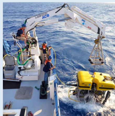
Hercules is recovered by operators on board the E/V Nautilus after a dive. Image courtesy of The Ocean Exploration Trust. http://oceanexplorer.noaa.gov/technology/subs/hercules/hercules-recover.html
